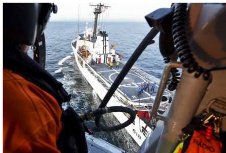
Coast Guard Aviation Electronics Technician 1st Class Chase Blackman handles a refueling hose that was hoisted to a MH-65 Dolphin during a helicopter in-flight refueling (HIFR) exercise near Newport, Ore., on Aug. 16, 2019. The aircrew executed this training mission with the crew of Coast Guard Cutter Active (WMEC 618) to ensure both units are properly trained when this situation arises during actual operations. (U.S. Coast Guard photo by Petty Officer 2nd Class Steve Strohmaier)
